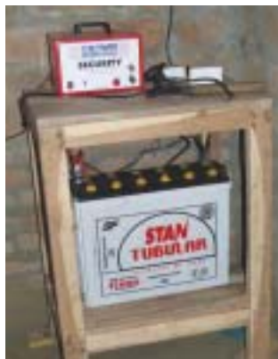
Energiser and battery
